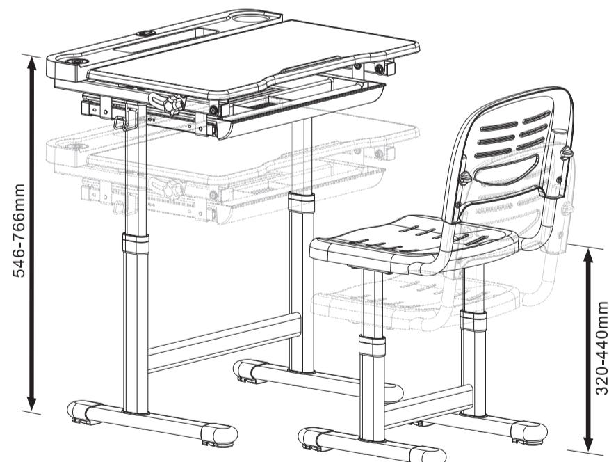
HOW TO ADJUST HEIGHT. Desk and chair can be adjusted by pulling up. Step on the support bar and pull up to the right height.
